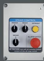
External control panel to command the belt cleaner functions
